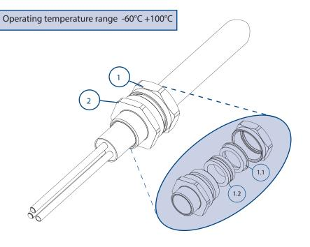
Certification Details Gland Type: 501/421 Exd IIC Gb, Exe II Gb, Extb IIIC Db Baseefa06ATEX0056X ঊ II 2 GD IP66 (€ IECEx BAS06.0013X IEx 14.0272X EAC TC RU C-GB.F605.B.00750 c CSA us No: 1015065 Class 1 Zone 1 AExd IIC, AExe II, Zone 21 AExtD Class 1 Div 2 ABCD, Class II Div2 Groups EFG, Class III
