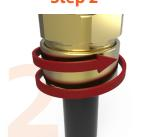
Tighten backnut until a seal is formed onto the cable, then tighten one further turn
